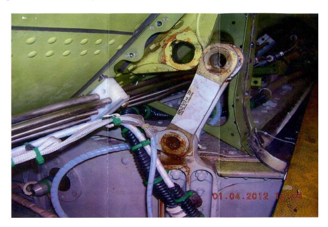
Hawker 800XP, Corroded Fuselage Attachment Links, ATA 5741
